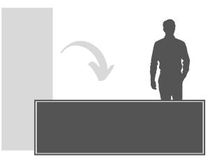
Starting at the top of the door, remove approximately 150mm of backing and press the brush strip firmly on to the metal frame in the centre.
