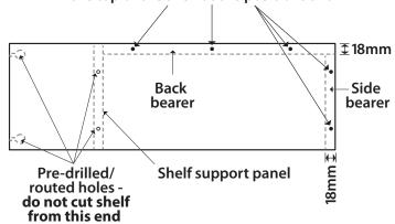
edge of the shelf support panel underneath. Then, ensuring the shelf is sitting firmly on both back and side shelf bearers, screw the shelf to the bearers using the 25mm screws provided and use the two M10 direct drive screws to secure the shelf to the shelf support panel through the pre-drilled holes. Finally, on the underside of the shelf, using a crosshead screwdriver, turn the minifix housings a quarter turn **anti-clockwise** to lock the shelf to the bolts on the divider panel.
