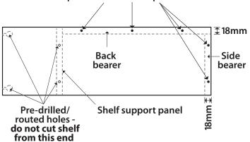
edge of the shelf support panel underneath. Then, ensuring the shelf is sitting firmly on both back and side shelf bearers, screw the shelf to the bearers using the 25mm screws provided and use the two M10 direct drive screws to secure the shelf to the shelf support panel through the pre-drilled holes. Finally, on the underside of the shelf, using a crosshead screwdriver, turn the minifix housings a quarter turn **clockwise** to lock the shelf to the bolts on the divider panel.
