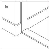
If you have a coving or cornice at ceiling level and you have ordered your system to fit to the ceiling height you must also remove the corresponding portion of the coving with clearance to allow for the wall liner to finish at ceiling level.
